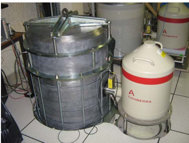
Fig. 5. The HPGe detector in passive shielding (left part) and the inner part of passive shielding (right part).
