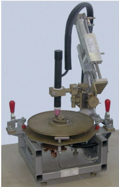
Fig. 1. The executing mechanisms unit and the technical characteristics of the installation for the remote welding of the thin-walled capsules.
